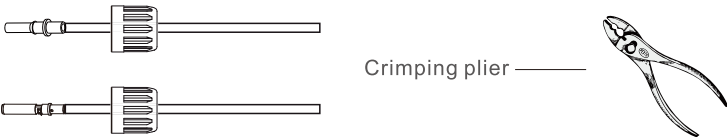
Pic 5.4 Crimp the contact pin to the wire
